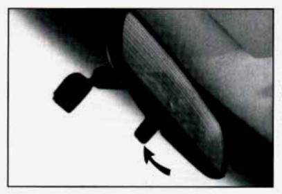
You can also adjust the mirror for day or night driving. Press the tab forward (away from you) for day driving. Pull the tab back (towards you) for night driving.
